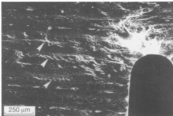
Figure 10 Enlarged view of part of Fig. 9 (CB33), showing the little cracks (arrowed) mainly restricted to the heavily mineralized region.
